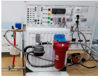
**Fig. 1. General view of the experimental setup for determining the efficiency of the acoustic-magnetic water treatment device**
